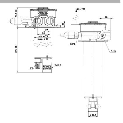
C = dismantling height required 220 mm
