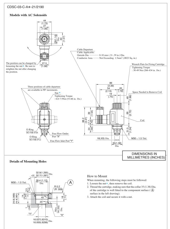
Note: The fitting portion of O-rings should have a good machined finish.
