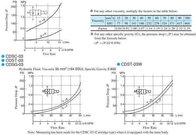
as the threaded connections and the gasket mounting type. • For any other viscosity, multiply the factors in the table below.
