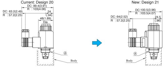
Note: The above drawings give illustrations for the cartridge type. The dimension A at the mounting section remains unchanged. In case of the Thread Connection Type and Gasket Mounting Type, a body is mounted to the hatched section. The dimensions of the body remain unchanged.
