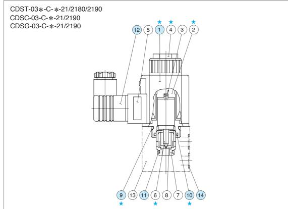
Solenoid assembly is composed of the parts marked with  $\bigstar$ .
